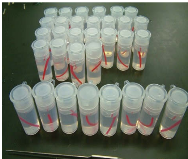
Fig. 1. Artificial blood vessel made of PVA for training [4]
