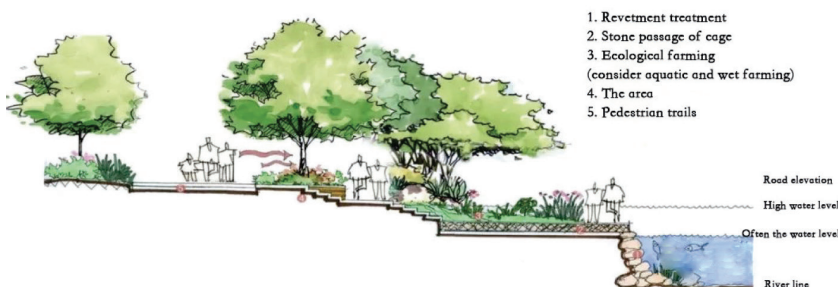
Fig. 6. Section structure of grassy slope step revetment
