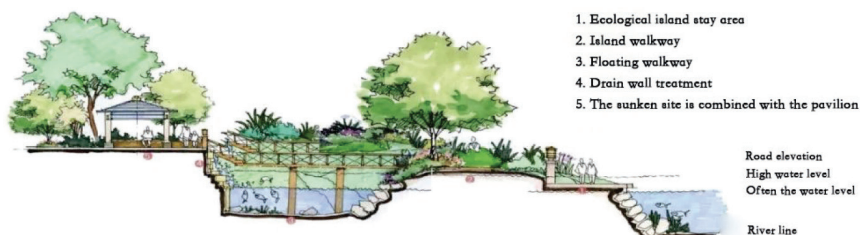
Fig. 8. Plank road and revetment section structure drawing
