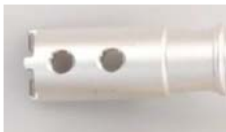
Fig. 6. Silver coated prosthesis module before implantation
