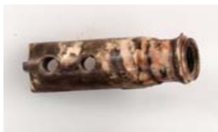
Fig. 7. Explanted silver coated module after a wear period of 3 years, tumor endoprosthesis was removed due to an aseptic loosening
