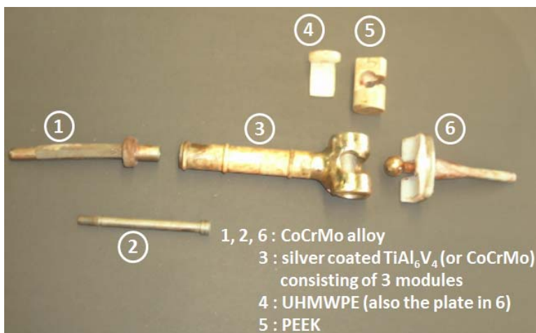
Fig. 4. Components of an explanted knee tumor endoprosthesis (after wear time of 3 years)
